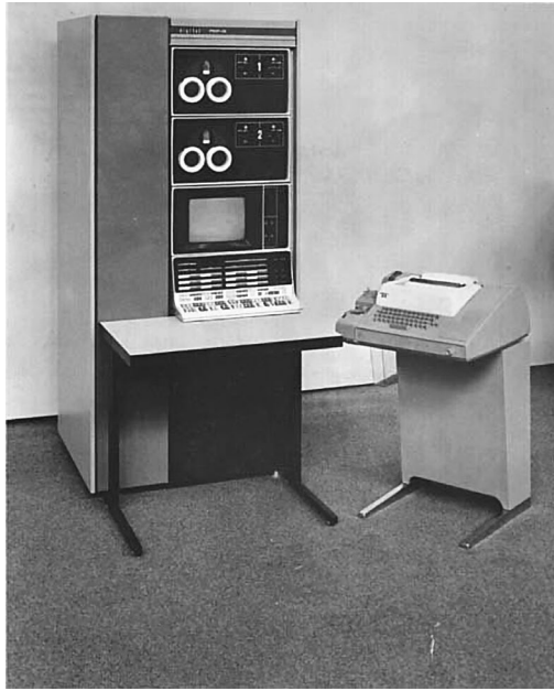
FIGURE 8.1. The PDP-12 computer produced by the Digital Equipment Corporation (ca. 1969). In the early 1980s, neurophysiologist Benjamin Libet used this device for carrying out his experimental studies of “mind time.” In contrast to earlier uses of computer technology in the psychophysiological lab, Libet applied the PDP-12 for calculating and storing experimental data as well as controlling the stimuli the test subject was exposed to in an adjoining room. Reproduced from PDP-12. User Manual , Carl Friend’s Mini-computer “Museum,” Reference Shelf, http://users.rcn.com/crfriend/museum/doco/PDP-12/index.shtml .
