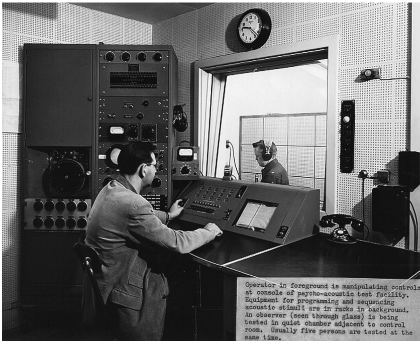
FIGURE 8.4. Psychoacoustic laboratory and control room in the Naval Electronic Laboratory (NEL), San Diego (ca. 1950). This is one of the rooms in which John Stroud, an electrical engineer, psychologist, and glowing cybernetician, carried out his experimental work on the “moment function” in human experience and behavior. The caption reads: “The operator in the foreground is manipulating controls at the console of psycho-acoustic test facility. Equipment for programming and sequencing acoustic stimuli are in racks in background. An observer (seen through glass) is being tested in quiet chamber adjacent to control room. Usually five persons are tested at the same time.” Reproduced from Navy Electronics Laboratory Historic Photographs , http://www.spawar.navy.mil/sti/publications/pubs/gen/nelhist/photos1.html .
